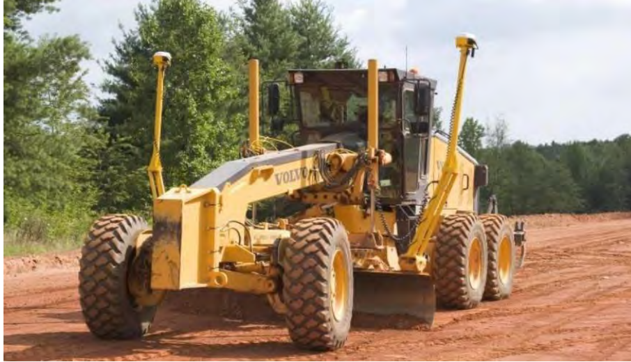
Grader equipped with AMG
