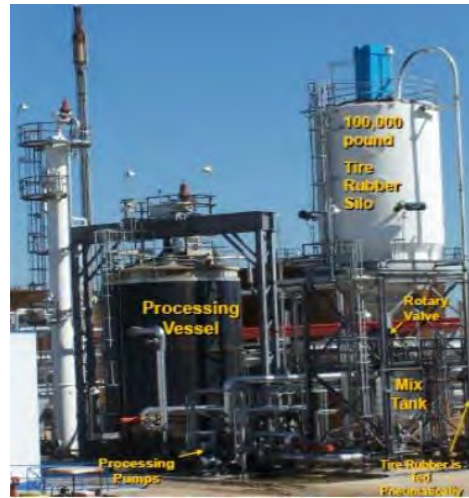
Terminal Blending Process for Rubberized Asphalt
