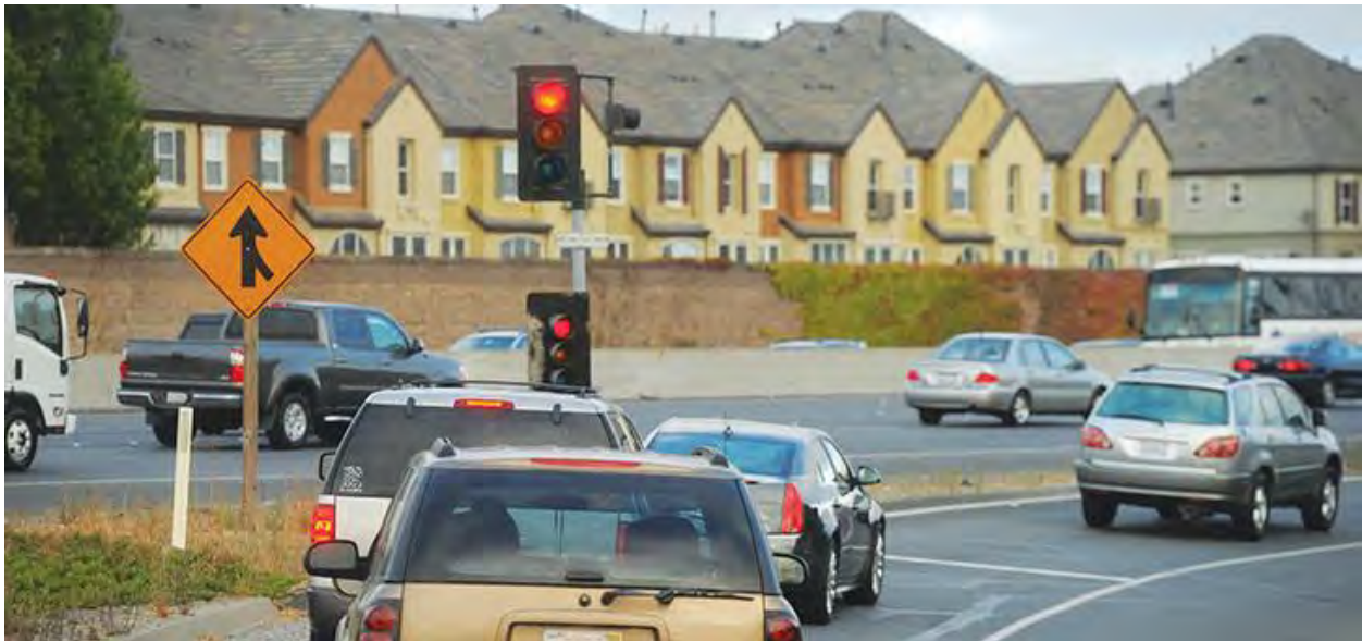
Bay Area Ramp Meter (source: MTC)
